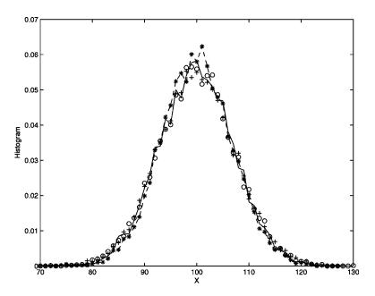
FIG. 1. Histogram (10 000 samples) of  $X_1$  solved by the SSA method (solid line), explicit tau (plot with "+"), implicit tau (plot with "\*"), and trapezoidal tau (plot with "o") for test problem (12) with  $\tau$ = 0.01.
