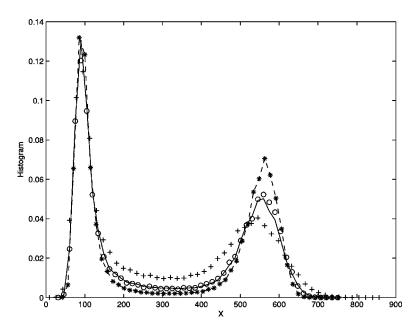
FIG. 5. Histogram (10 000 samples) of  $X_1$  solved by the SSA method (solid line), explicit tau (plot with "+"), implicit tau (plot with "\*"), and trapezoidal tau (plot with "o") for Schlögl reaction with  $\tau$ =0.4.
