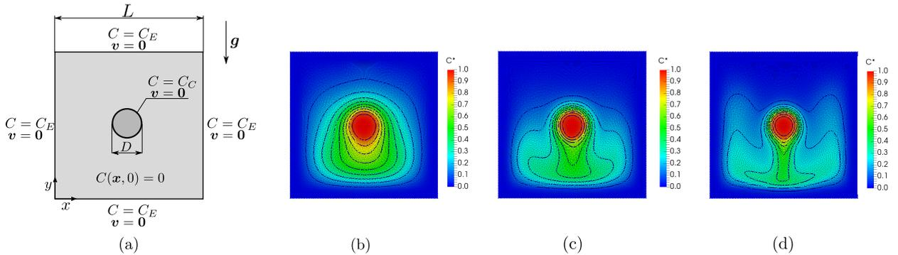
Fig. 4. (a) Schematic of natural convection in a cylinder inside a square enclosure. (b), (c) and (d) show isocontour plots of dimensionless concentration  $C^*$  at steady-state, for (b)  $Ra = 10^4$ , (c)  $Ra = 10^5$  and (d)  $Ra = 10^6$ . Results shown in (b), (c) and (d) were interpolated using a Gaussian kernel, for clarity purposes.
