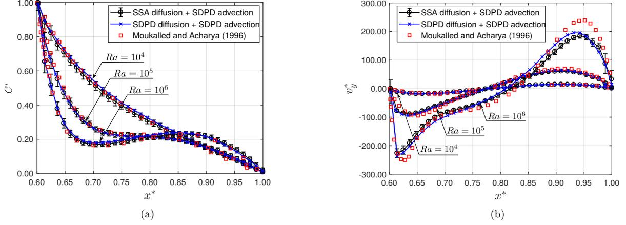
Fig. 5. (a) Comparison of the mean dimensionless concentration ( $C^*$ ) and (b) dimensionless (re-scaled by  $\sqrt{Ra/Sc}$ )  $y$ -velocity ( $v_y^*$ ) centerline profiles, for  $Ra = 10^4, 10^5$  and  $10^6$ , computed at  $t = 50$ , over  $N_r = 100$  realizations.
