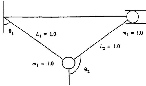
FIG. 5.5. Example 5.2, slider-crank mechanism.
