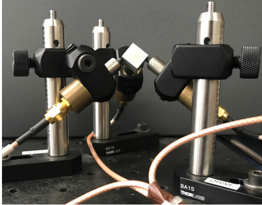
Fig. 3—Photo of a parallelepiped specimen positioned on the piezoelectric transducer cradle prior to a broadband RUS measurement.
